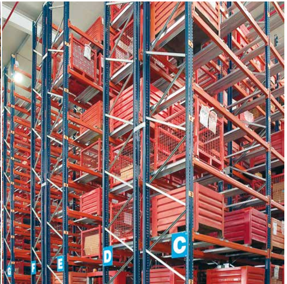
Selective pallet racking system with metal containers
